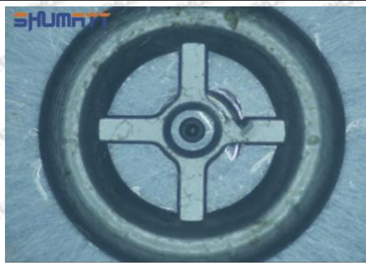
The misalignment of the semi ball causes damage to the orifice plate when installing it
