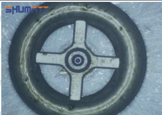
The wear of the middle oil back-flow hole causes gap between semi ball and orifice plate, and causes the orifice plate to be washed out by high-pressure oil
